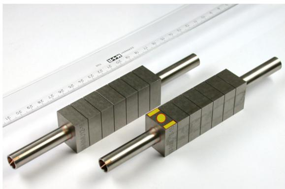
**Fig. 1.** Examples of ITER W monoblock mock-ups HHF tested in GLADIS. Seven monoblocks of  $23 \times 28 \times 12 \text{ mm}^3$  are bonded onto a cooling tube made of CuCrZr. For one W monoblock, the ROIs for the IR analysis are marked in yellow.
