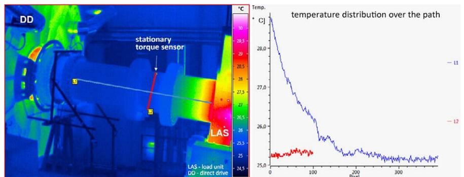
Temperature distribution of the torque transducer of the 4 MW wind turbine test bench of RWTH Aachen University
