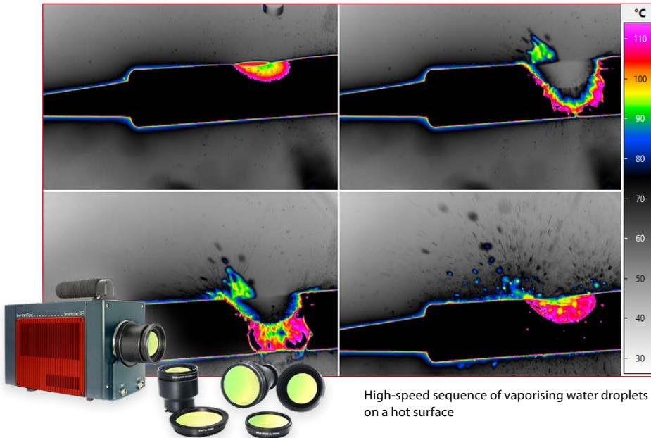
High-speed sequence of vaporising water droplets on a hot surface
