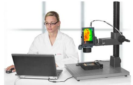
Lock-in Thermography package with VarioCAM® HDx and IRBIS® 3 active software
