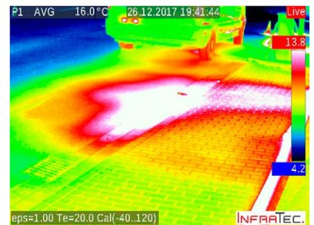
The image was captured due to damage that led to water losses in the district heating network. Using an infrared camera, the damage to the connection pipe for the district heating could be located quickly and accurately.
