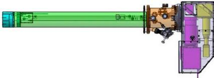
Snapshot of CAD model of high-resolution IR/VIS prototype endoscope. The IR and visible cameras are mounted at the end of the endoscope via holder
