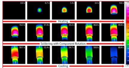
Process sequence for Laser High Temperature Capillary Gap Soldering of a tube-plug-in connection
